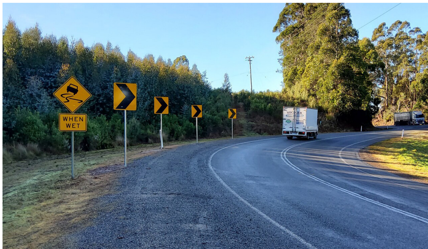
Motorcyclist safety can be improved through hazard warning signage.
